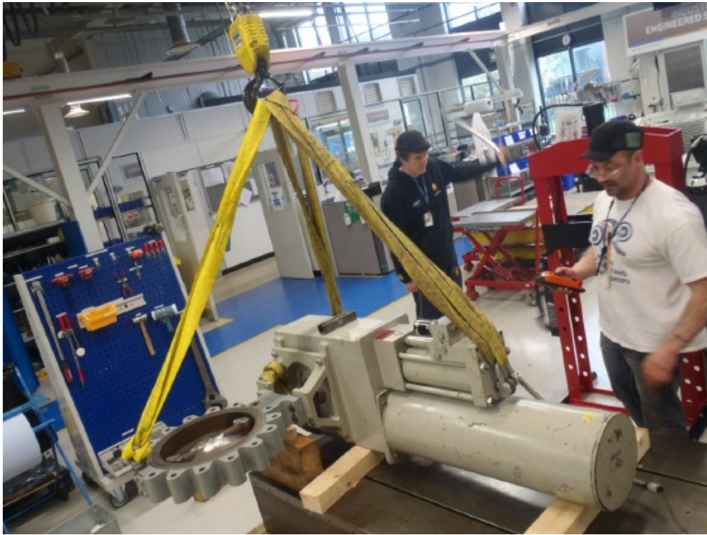
Moog technicians positioning actuator for disassembly
